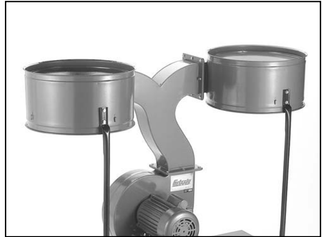
Figure 13. Collector rings installed.
